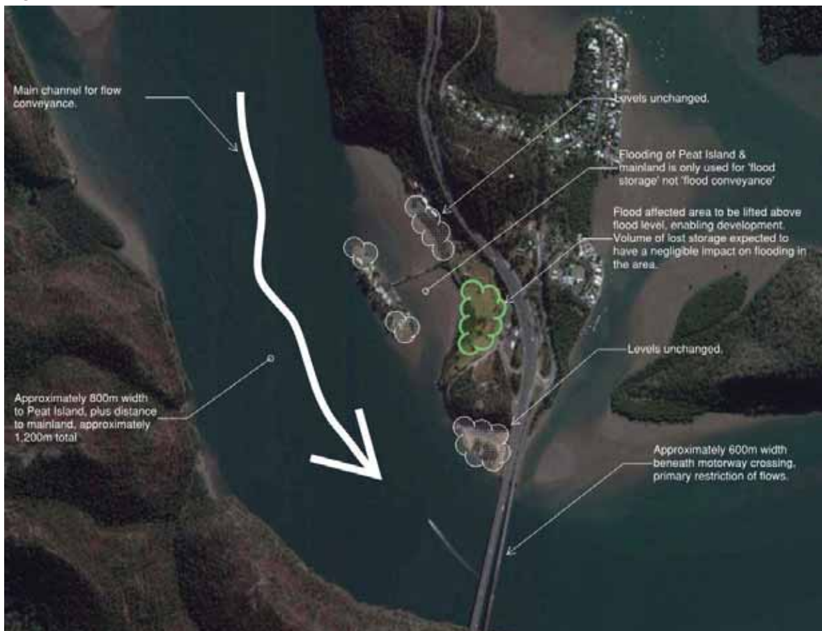
Figure 6: Flood Characteristics Across The Site
